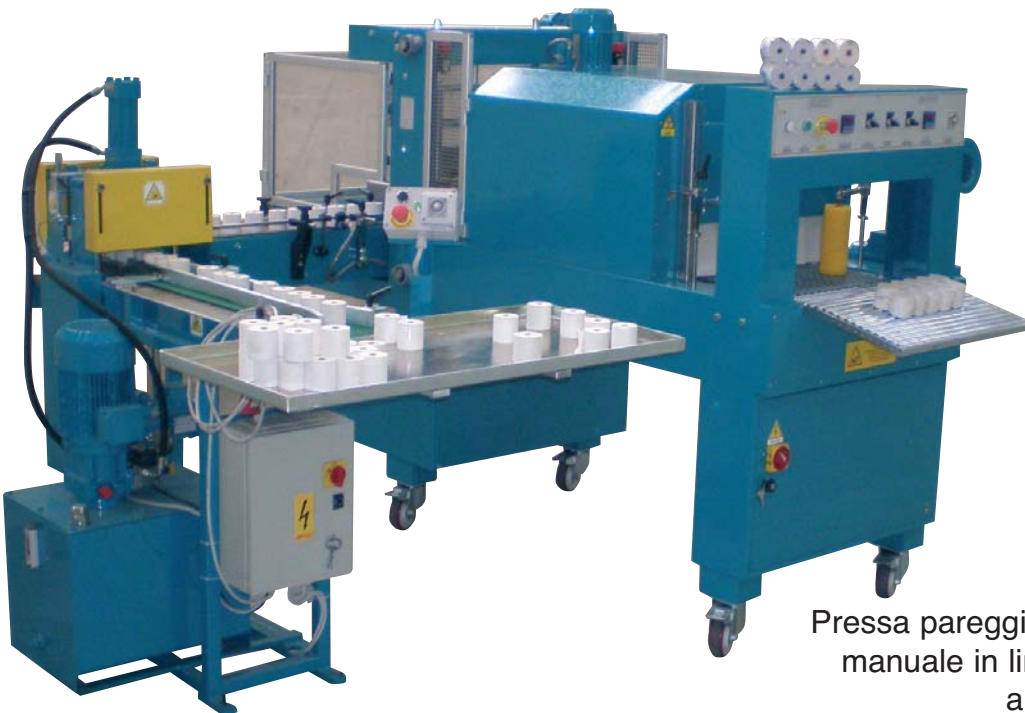
Press machine for rolls with manual feeding and automatic shrink wrapping
